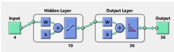
Figure 12: Two-Layered Feed Forward Network
