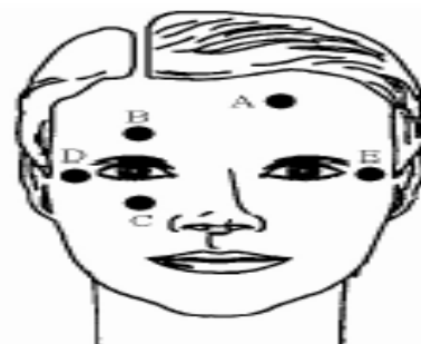
Figure 9: Placement of electrodes for EOG recording [6,7,8,10,21,22,32,48,50,52]
