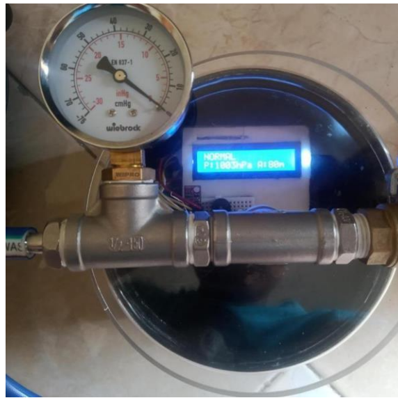
Fig. 3 Prototype Cabin Altitude Warning Switch Status Normal
