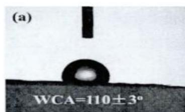
FIGURE 3. Pure PP cross-sectional surface
