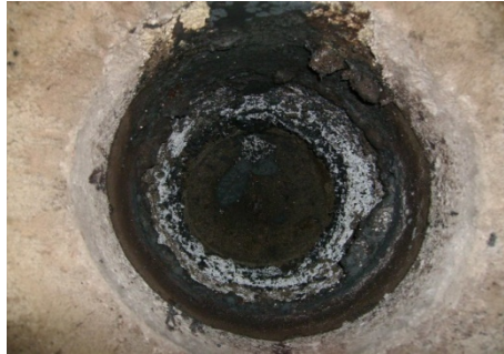
Figure 13. Lining Condition after Third Time Melting
