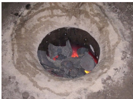
Figure 11. Preheating the Furnace
