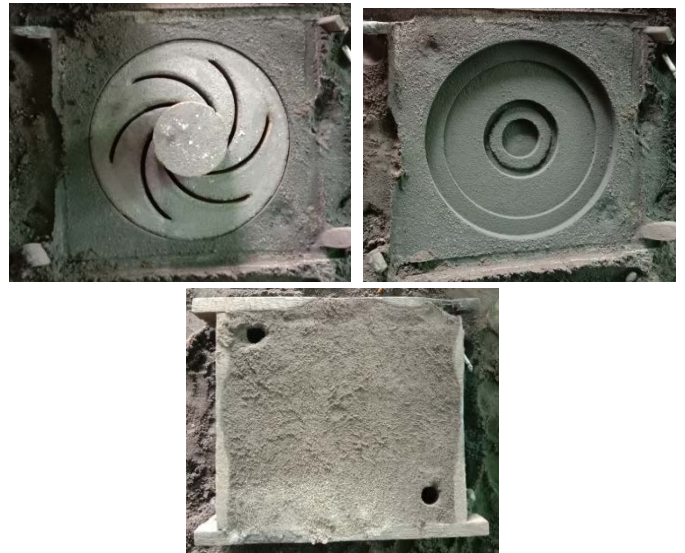
Fig 8. Mould Making and Sand Casting for Impeller
