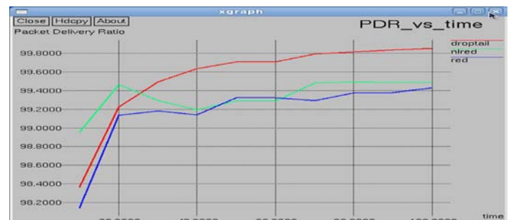
Figure 12: Comparing Variation of Packet Delivery Ratio (PDR) for Drop Tail, RED and NLRED
