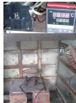
Fig 3.5 SnO 2 :F coating by spray pyrolysis
