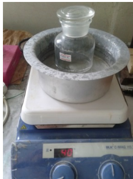
Fig 3.3 SnCl 4 .5H 2 O solution in water bath at 40°C
