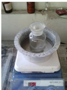
Fig 3.4 Mixed solution SnCl 4 .5H 2 O and NH 4 F in water bath at 60°C
