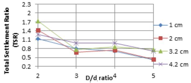
Figure 3 b TSR VS D/d Ratio for soaked condition
