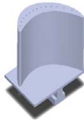
Fig4. Turbine first stage rotor blade with 13 holes
