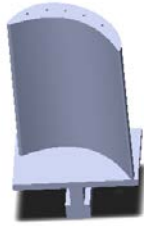
Fig2. Turbine first stage rotor blade with 5 holes
