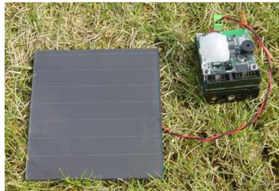
**Figure 1. Solar panel connected to Sensor Board**
