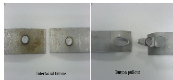
Figure 7: Weld failures produced by the force profiles
