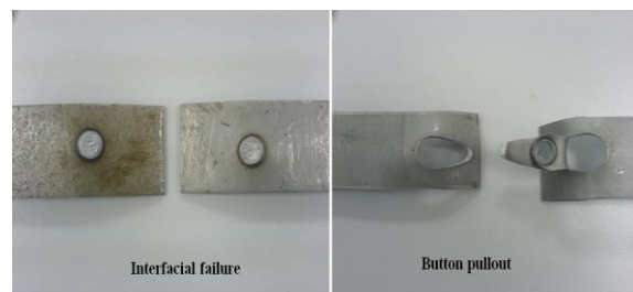
Figure 7: Weld failures produced by the force profiles
