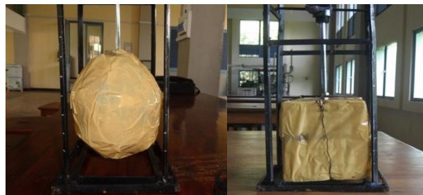
Figure 16: Designed and Fabricated Spherical and Cubic Shaped Buoyancy
