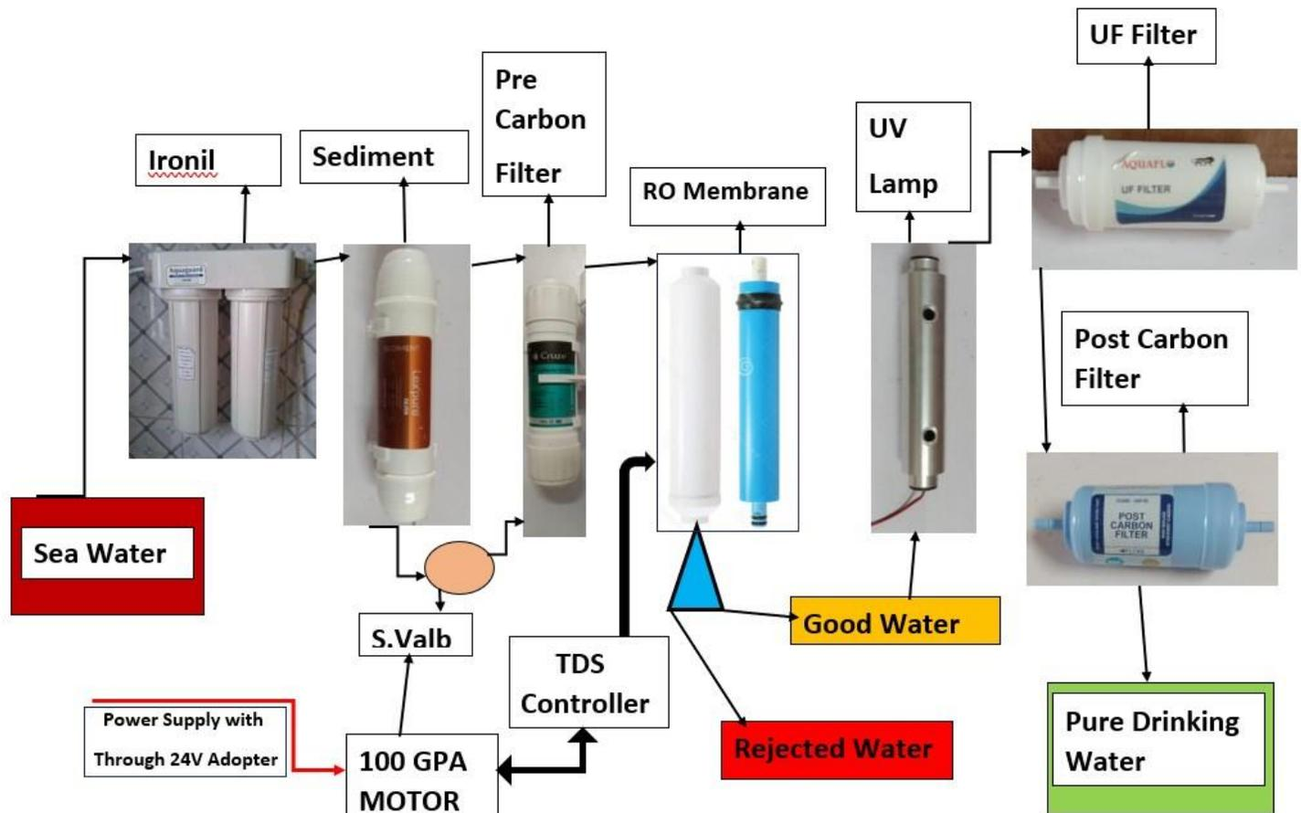
Figure 1 Schematic Layout of the desalination unit
