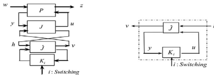
Fig.3. The proposed control structure and  $Q_0 = F_l(\hat{J}, K_i)$
