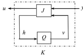
Fig.2. parameterization of  $\gamma$ -suboptimal controller with  $Q$ .
