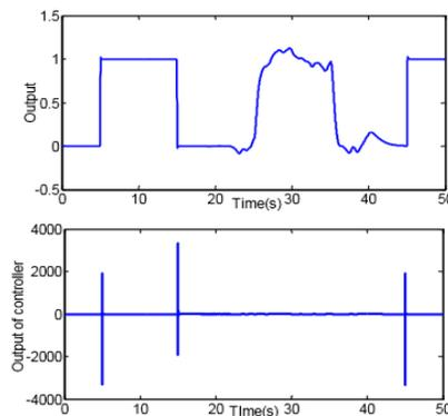
Fig.7. The switching strategy between stabilizing controllers
