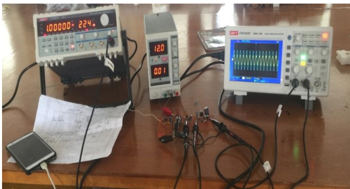
Figure 10: Test Output of Power amplifier and Power Supply Generator on Universal Card
