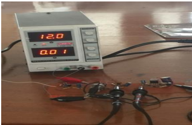
Figure 9: Test Output of Power amplifier and Power Supply Circuit on Universal Card
