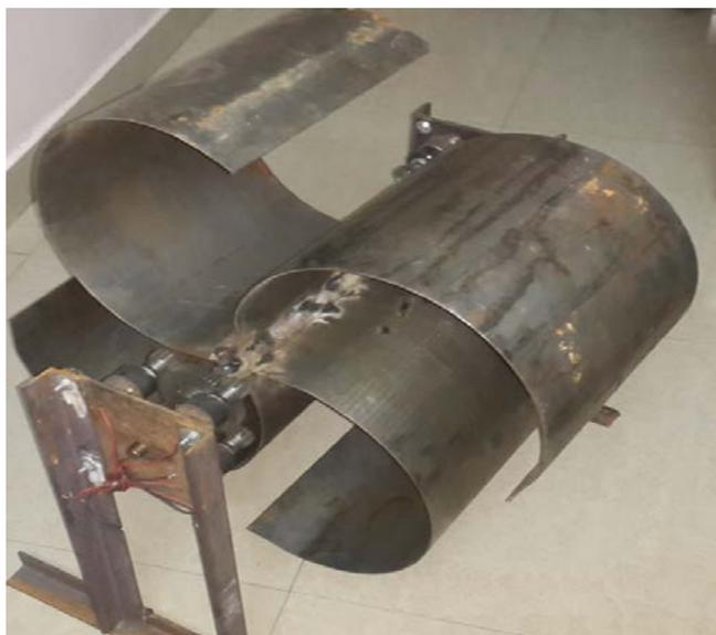
**Fig.5 Advance Hybrid Savonius With Arm Gear Based Structure model**
