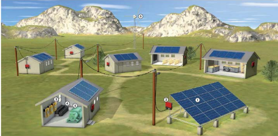
Fig. 1.4: Expansion options of an AC coupled hybrid system for a village electricity supply
