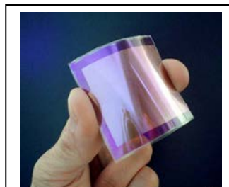
Fig. 6: A Painted Flexible Coloured Solar Cell
