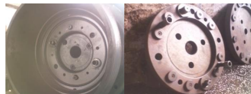
Fig.2.1.4 Finishing operation setup and lathe fixture
