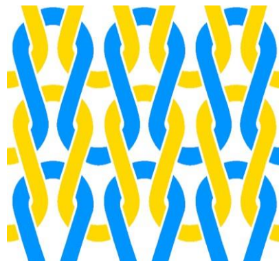
Figure 1. Structure of a single jersey knitted fabric
