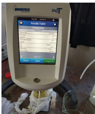
Fig 6: Determining viscosity using Brookfield Viscometer DV2T
