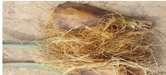
Figure1: Date palm petiole with the mechanically extracted date palm petiole fiber (DPPF)
