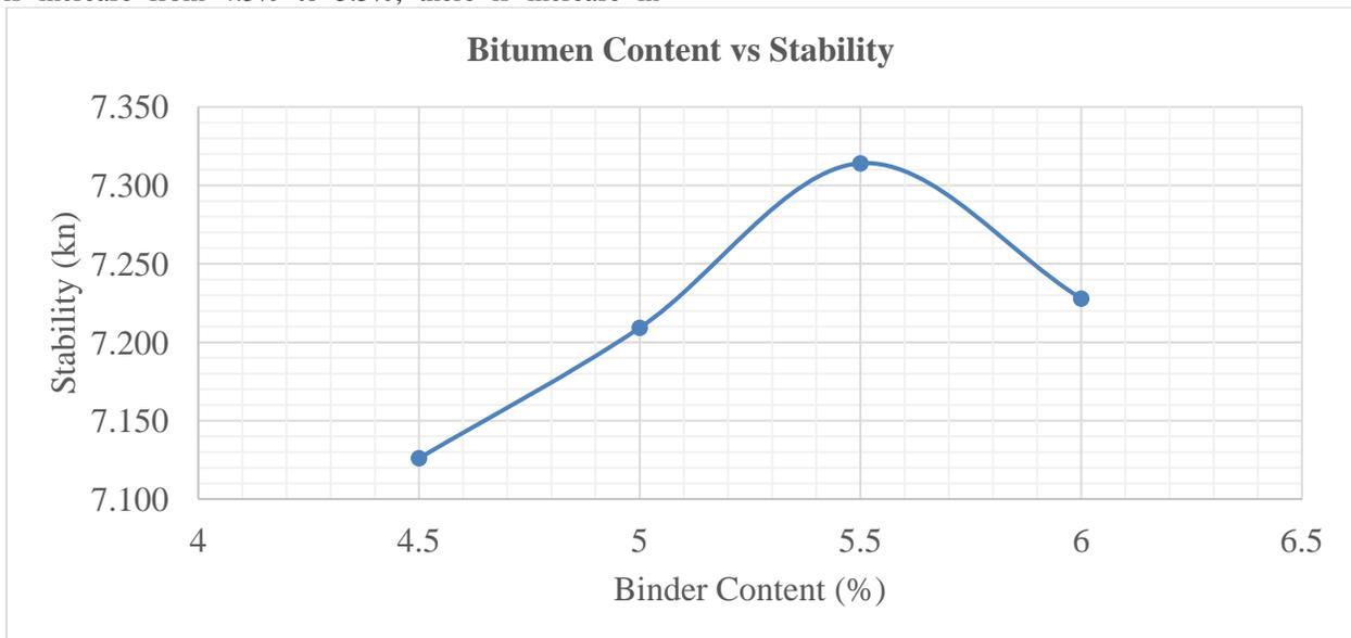
Figure 2(b): Bitumen content vs stability.
