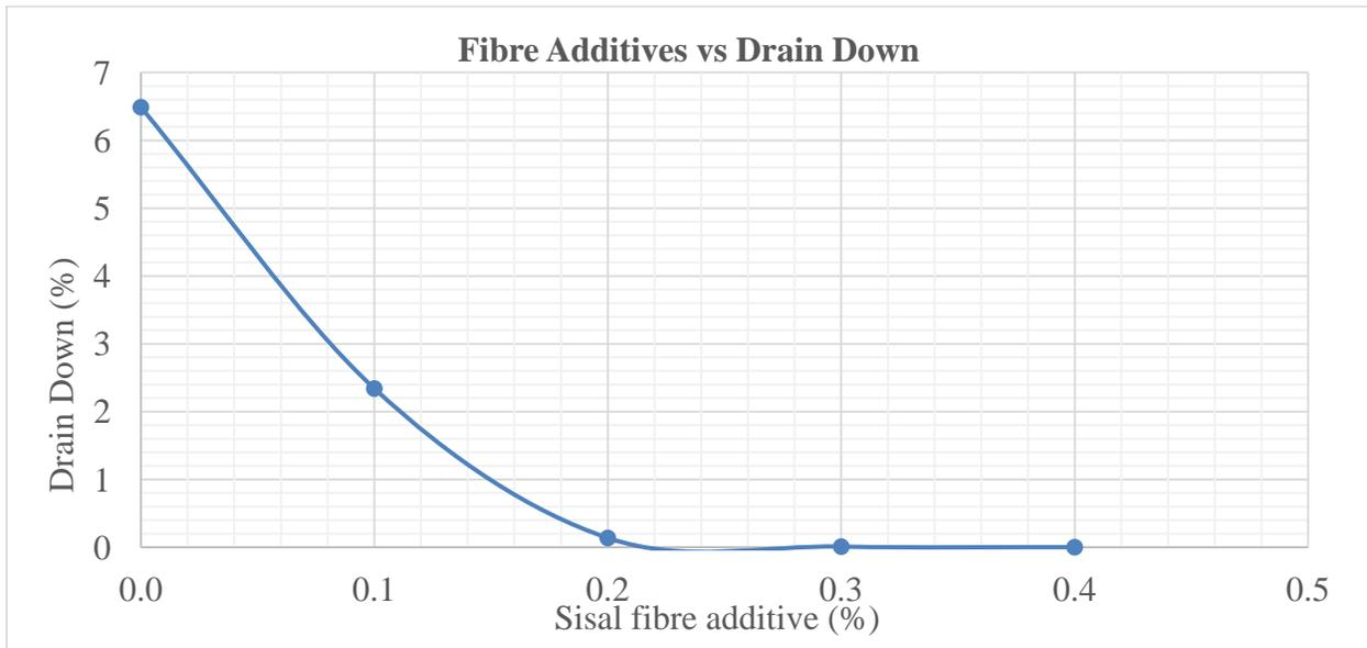
Figure 3: Variation of drain down with different percentages of SF.
