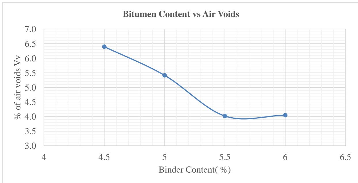
Figure 2(c): Bitumen content vs % Air voids
