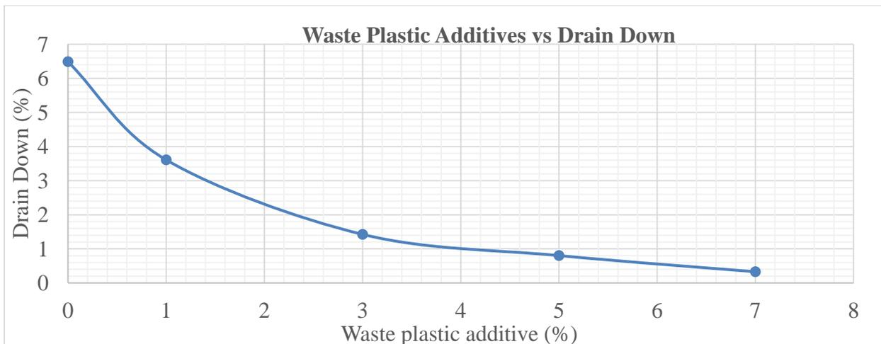
Figure 4: Variation of drain down with different percentages of waste plastics.
