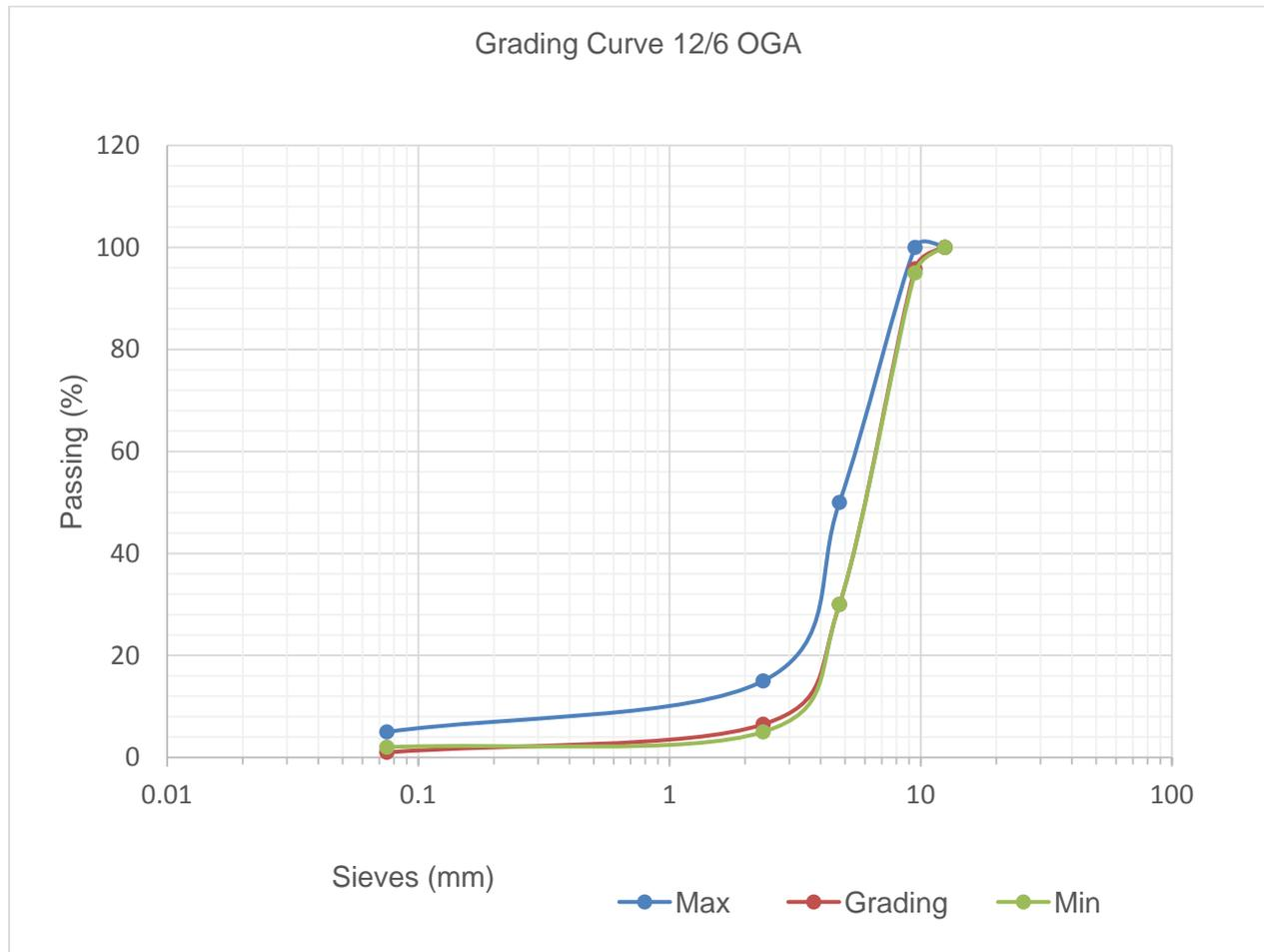
**Figure 1: Grading curve for 12/6 mm aggregate for OGA mix.**
