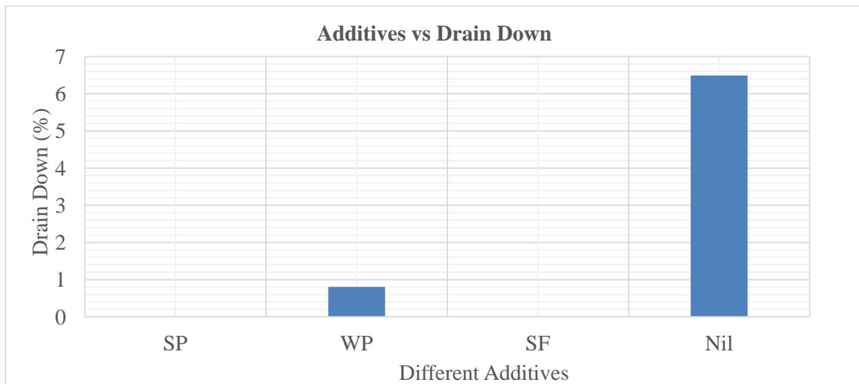
Figure 4: Drain down results for different additives
