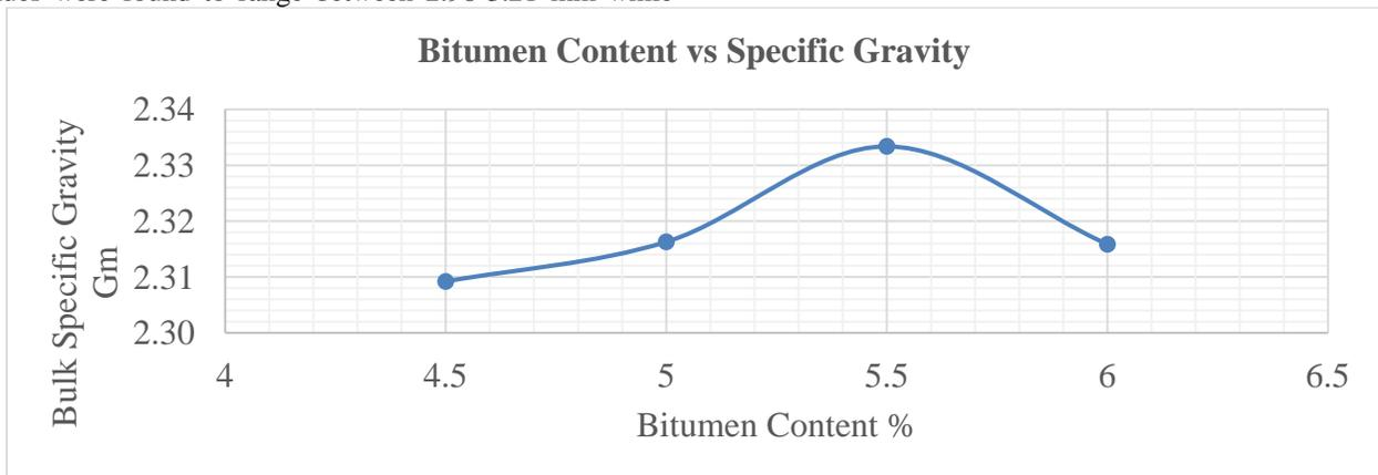
Figure 2(a): Bitumen content vs density of mix.
