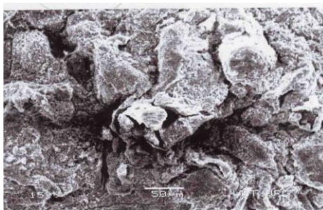
Figure 13 (a): SEM micrographs of jatropa curcas -calcium alginate beads before adsorption
