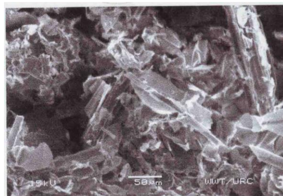
Figure 12(a): SEM micrographs of bagasse-calcium alginate beads before adsorption
