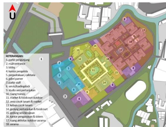
Fig. 2. Massing organization based on area: public and administration (blue); working and interaction (yellow); private and dormitory (red); service (purple)
