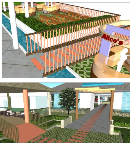
Fig. 5. Above: physically boundaries but visually accessible access for autistic individual in working area. Below: the color of pathways pattern used as signage
