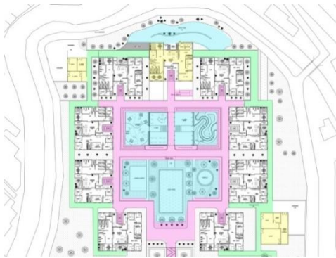
Fig. 4. Simple linear circulation arrangement of dormitory area: autistic individual (pink); service (green); supervision spot (yellow); outdoor communal space (blue)
