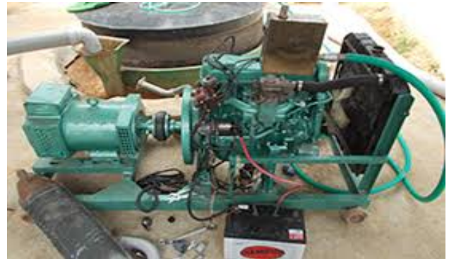
Plate 10, Methane Operated Engine[23].
