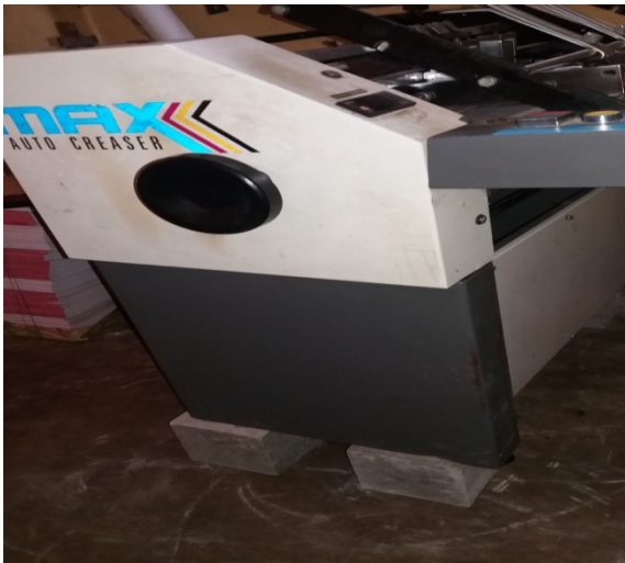
A medium weight machine placed above the compound concrete blocks with loading surface on waste rubber.
