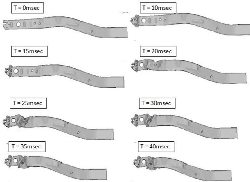
This is the front longitudinal member for which thickness variation is done to study the effect of variable thickness. This member is gradually deformed during the crash event initiating a collapse at 25 msec. Maximum resistance is offered before the collapse is function of thickness, geometry and material.
