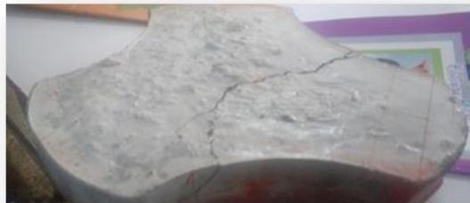
**Figure 3.20 paving block after flexure testing**
