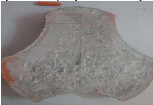
**Figure 3.19 Paving block before flexure Testing**
