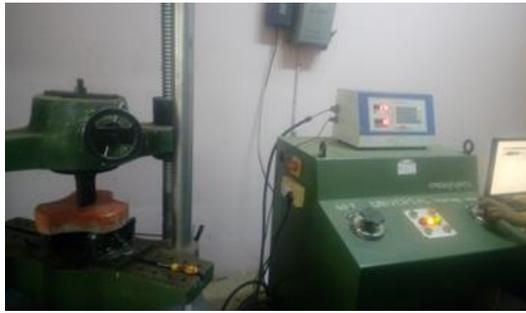
**Figure 3.18 Flexural Testing on Paving Block.**
