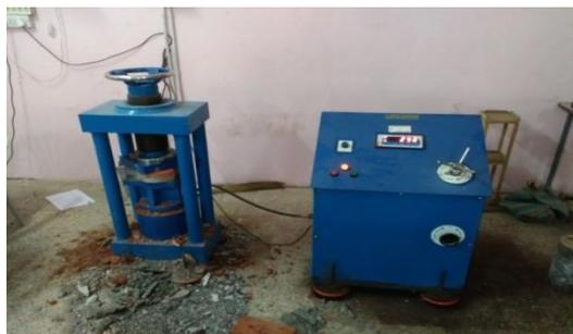
**Figure: 3.15 Compressions Testing On Paving Block**
