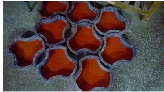
**Figure 3.6 C-Type Rubber Mould.**
