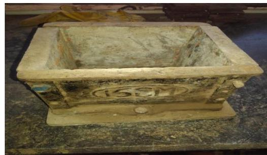
**Figure 3.7 Concrete Cube Mould**
