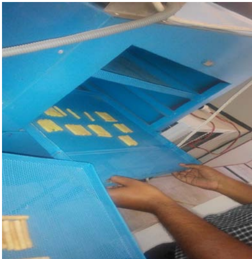
Figure 10: Drying chamber trays
