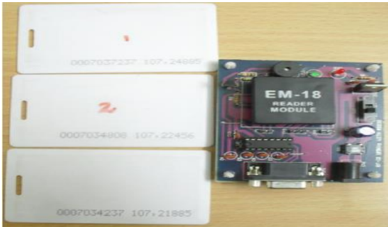
Fig3. RFID reader and tag.
