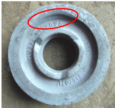
Photograph 1: Unfilling defect at front side of job
