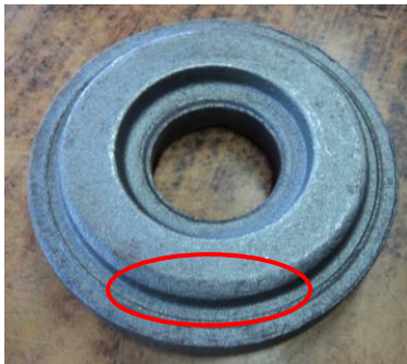
Photograph 2: Unfilling defect at back side of job
