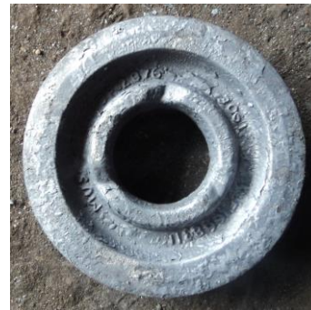
Photograph 5: Defect free job
