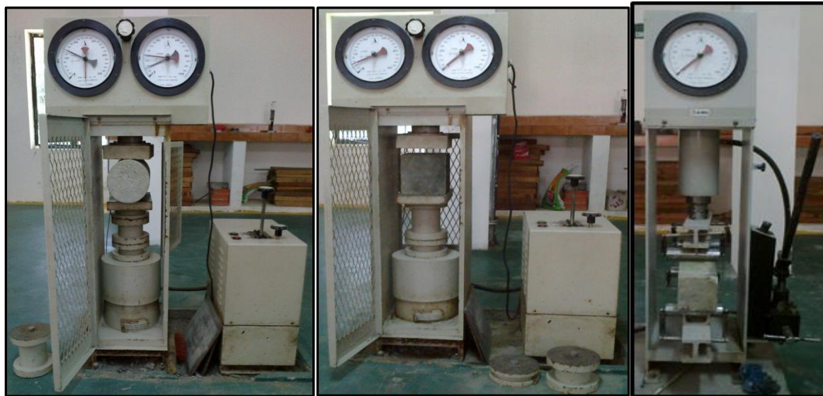
Figure 4: Testing of Specimens in Compression Testing Machine & Flexural Strength Testing Machine
