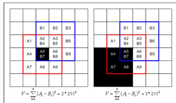
fig(1) Measuring the intensity Variation by using 3×3 window
