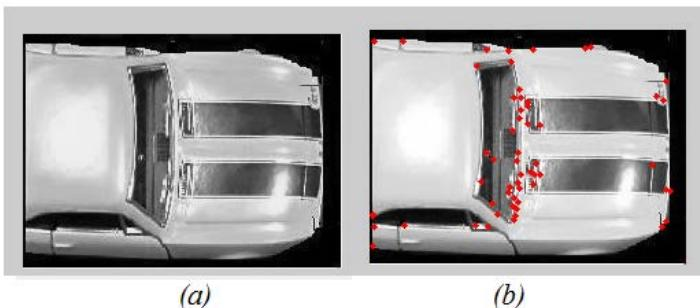
fig (13) Detecting corners and sharp curvature
