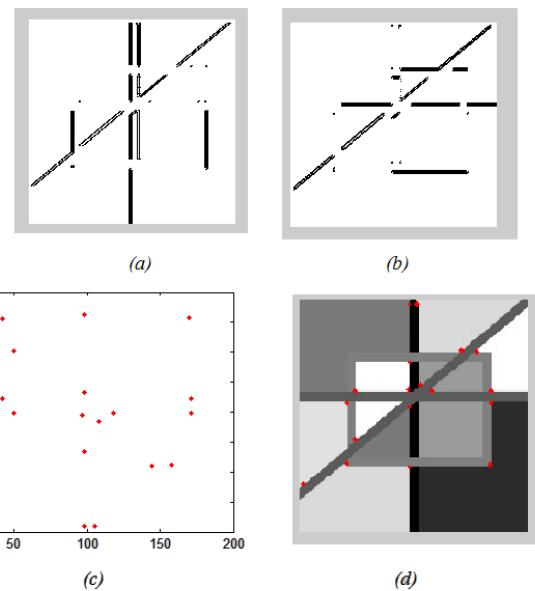
fig(10) (a) the pixels with horizontal gradient x-direction (b) the pixels with vertical gradient y-direction (c) distribution of corner points (d) localization of corners detected as final result
