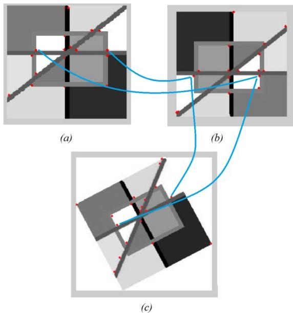
fig(14) Detecting corners under rotation situation
