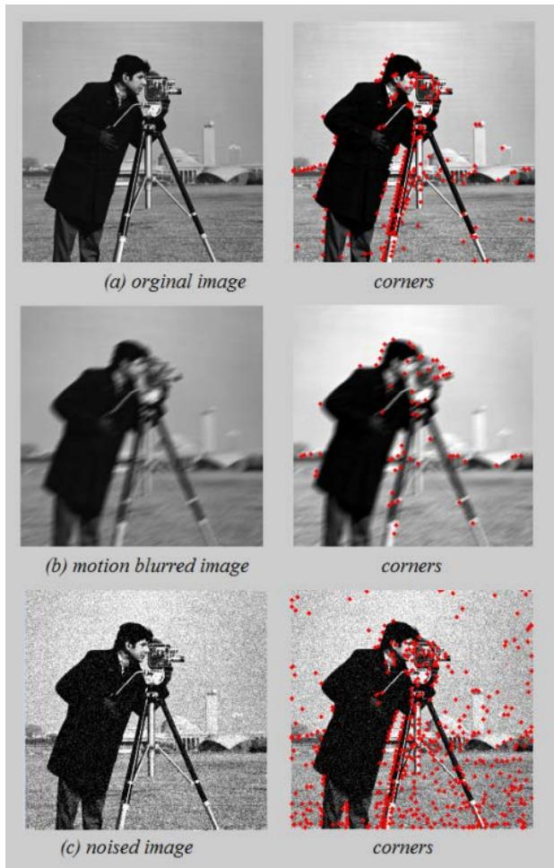
fig(12) More examples for detecting corners in : (a) normal image (b) blurred image (c) noised image
