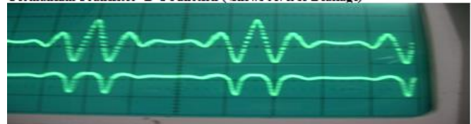
Fig. Germanium Transistor B-C Junction ( Shows reverse Leakage)
