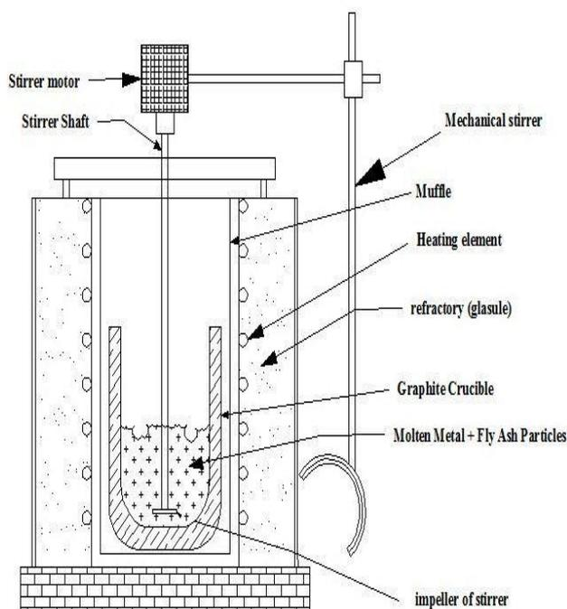
**Figure2. Experimental set-up for preparation of composite**
