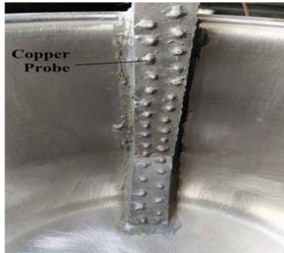
Figure 6: Water level sensor probes.
