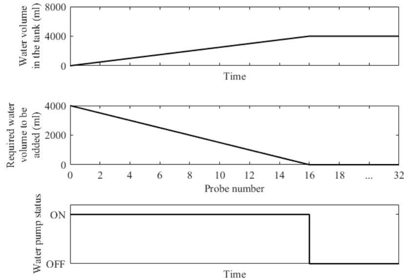
Figure 7: (a) desired water level in the pot, (b) the relationship between the required water volume to be added and the signal probes and (c) logic representation of the water pump operation time.
