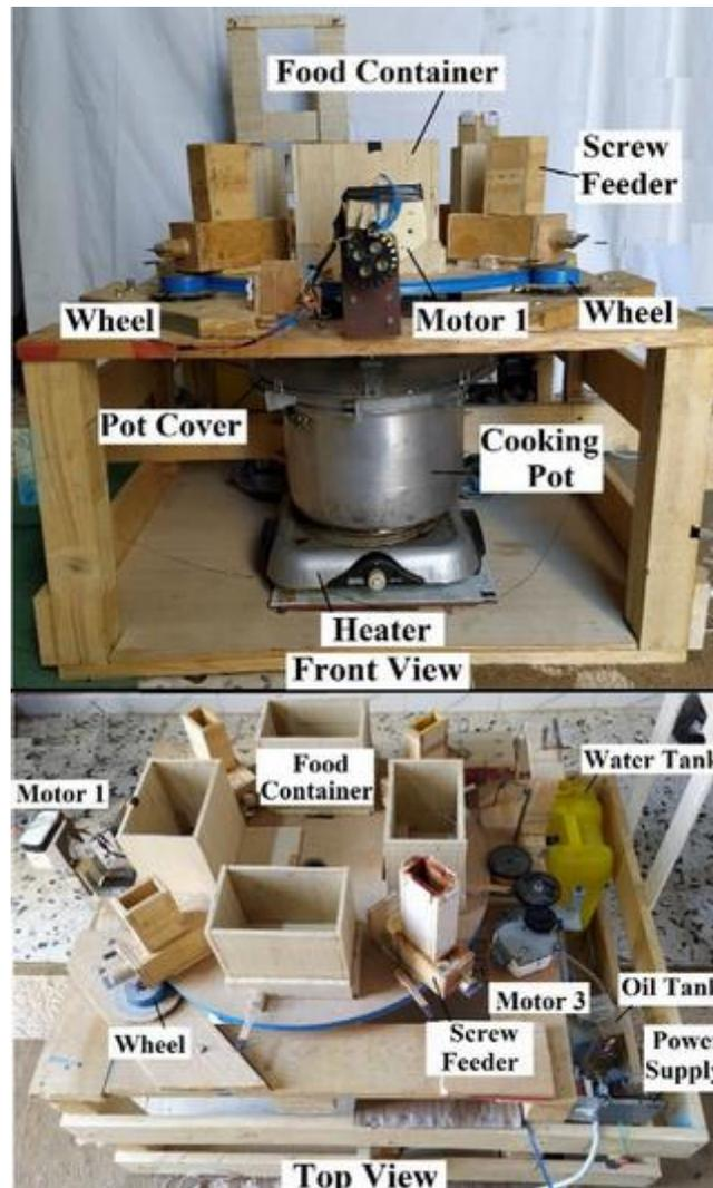
Figure 1: The general structure of the system with all elements and taken from different views.
