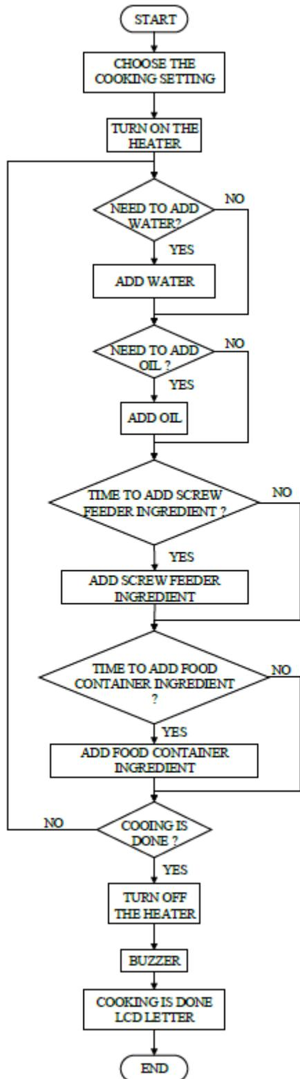
Figure 2: System operation flow chart.
