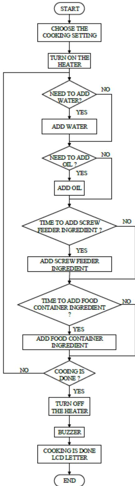
Figure 2: System operation flow chart.
