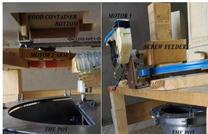
Figure 4: (left) Rotating the screw feeder, (right) opening and closing the feed container.
