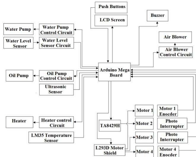
Figure 2: General block diagram of the system
