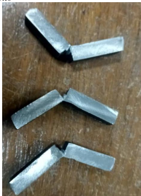
Figure 2b: Failure after impact Test
