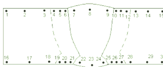
Figure 1. The Welded sample showing the 30 points at which the hardness measurement was made
