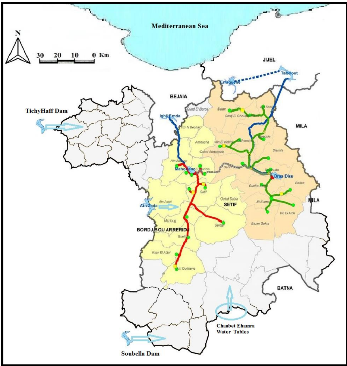
Figure 4: Main water supply systems in Setif Province [21-23],
