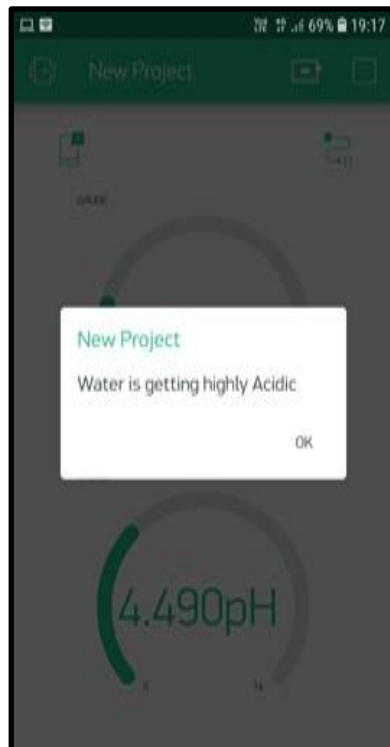
Figure 5: An alert message on user's android application wherein as soon as the water goes below 5.5, this message gets displayed.
