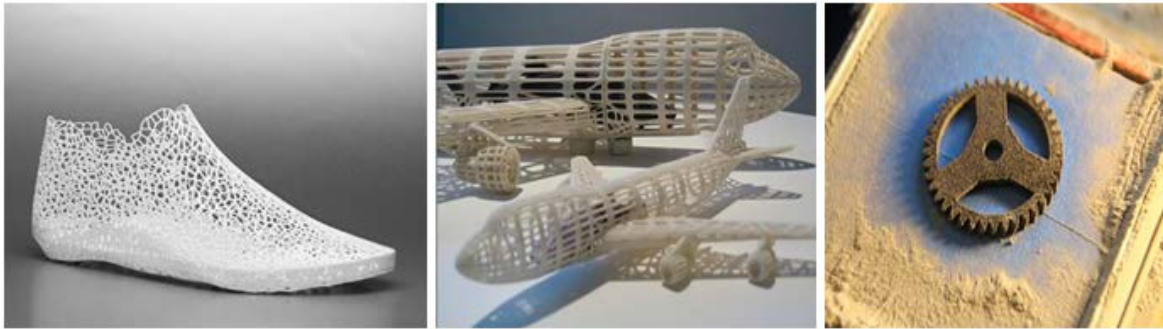
Figure 7: Parts printed by SLS
