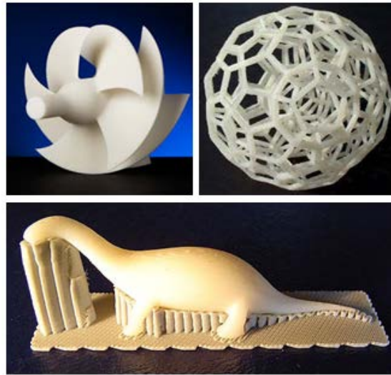
Figure 5: Typical objects printed by FDM
