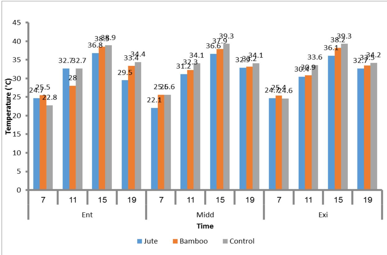
Fig. (1) Temperature at different time on the three traditional stores.
