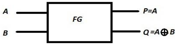
2(a) Block diagram of 2 input Feynman gate
