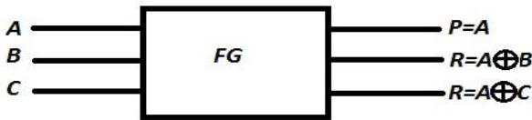
2(b) Block diagram of 3 input Feynman gate
