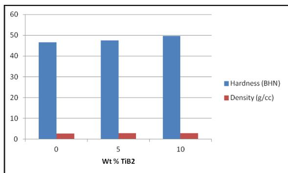
**Figure 6. Density and hardness of TiB<sub>2</sub>/Al MMCs.**
