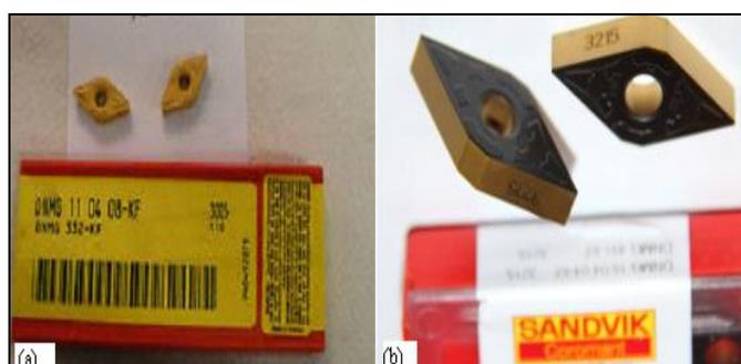
Figure 2: (a) SANDVIK: DNMG 3005 Tool (K<sub>10</sub>)
