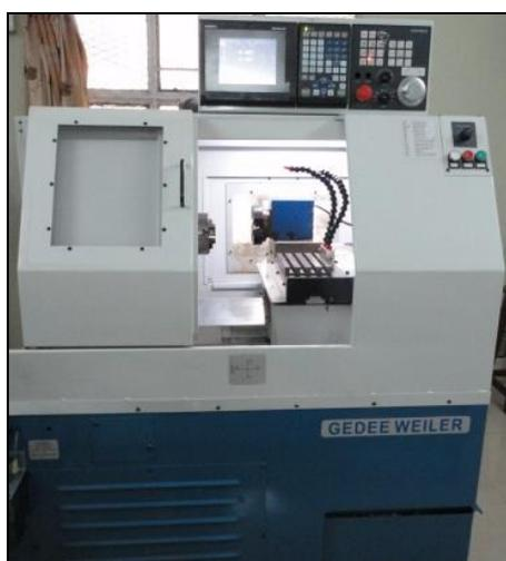
Figure 1: CNC turning center. (MITSUBISHI-EZ Motion NC E60)
