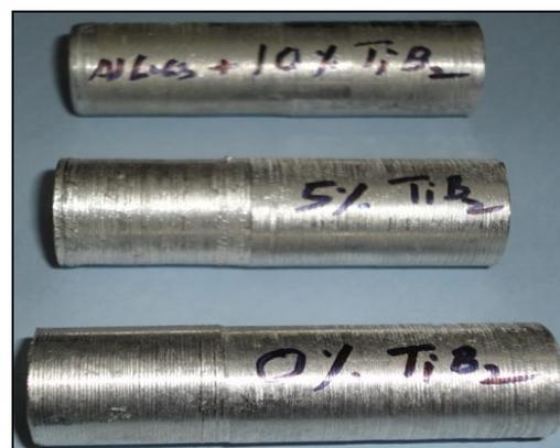
Figure 3: Composite Material 0, 5 & 10 wt%TiB<sub>2</sub> Reinforced with Al-6063.
