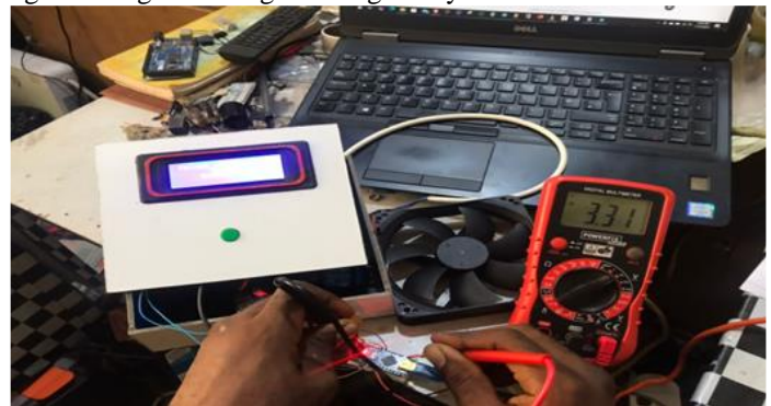
Figure 10. Buzzer Voltage when Helmet was not Recognized
