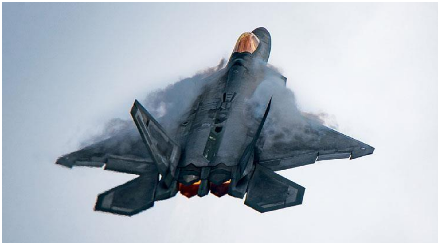
Figure: In the F-22 Raptor, reflections were reduced when the leading edge of the wing and the tail plane were positioned at the same angle. [6]
