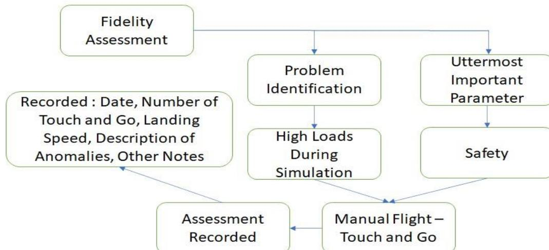
Figure 1. The Methodology for Fidelity Assessment of Boeing 737-800 Simulator
