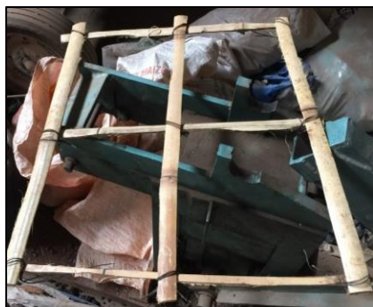
Figure 4: (A) Bamboo slab reinforcement; (B) Bamboo slab line loading arrangement
