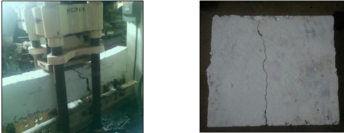
Figure 6: (A) Beam failure mode and, (B) Slab failure mode
