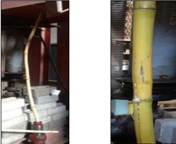
Figure 5: (A) Dry bamboo sample under compression testing; (B) Failed bamboo showing split of the stem following buckling
