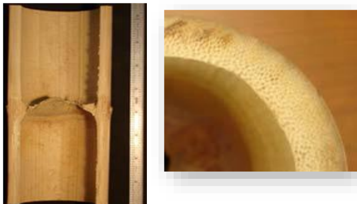
Figure 2: longitudinal and transverse sections of bamboo culm
