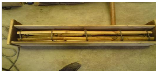
Figure 3A: Beam reinforcement arrangement
