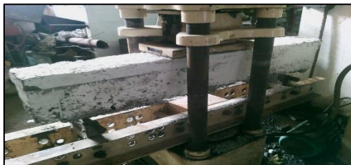
Figure 3B Three point beam loading arrangement
