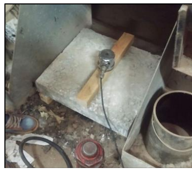
Figure 4: (A) Bamboo slab reinforcement; (B) Bamboo slab line loading arrangement
